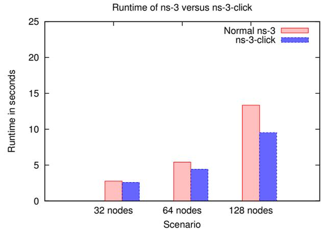
**Figure 7: Average wall clock running time of ns-3 versus ns-3-click for running an IP Router configuration. Results indicate that ns-3-click benefits from improved running time by performing Layer 3 functionality in Click.**
