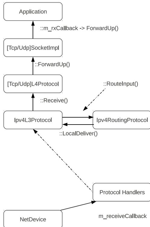
**Figure 4: Path of packet going up the stack in ns-3.** The packet flows along the upward arrows, with the protocol handler passing the packet to either the ARP instance or the IP layer (shown above), depending on the packet type. Forwarding decision is made at Layer 3 using a *RouteInput()* query to the routing protocol instance.
