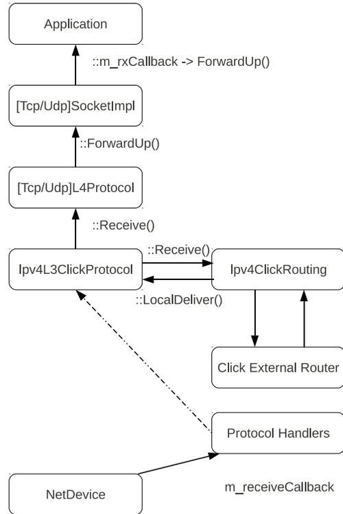
**Figure 6: Path of a packet going up the stack in ns-3-click.** *ns-3-click* handles all Layer 3 functionality including ARP via Click itself, so the protocol handler always passes packets up to *Ipv4L3ClickProtocol*. Instead of a call to *RouteInput()* as in Figure 4, the forwarding is performed by passing the packet through the Click graph.
