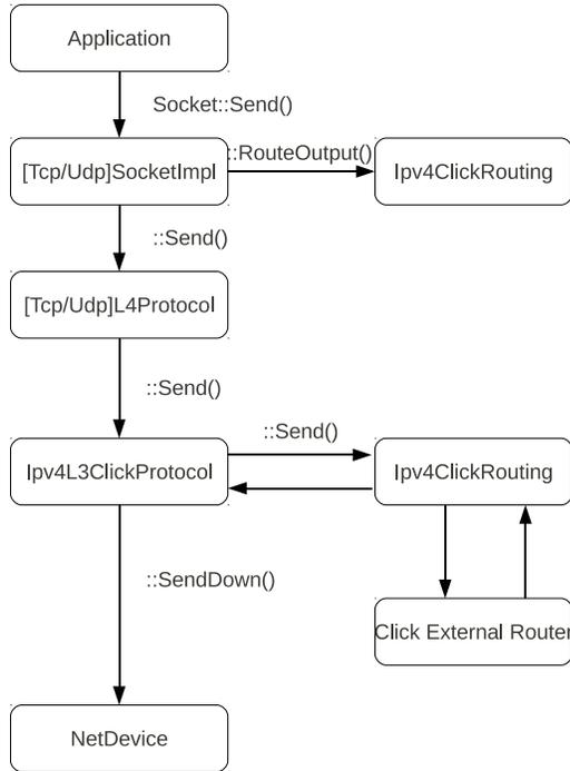
**Figure 5: Path of a packet going down the stack in ns-3-click.** The flow is similar to Figure 3 except at Layer 3, where the packet is actually passed to the Click router and back via *Ipv4L3ClickProtocol* and *Ipv4ClickRouting*, so as to have the packet traverse the Click graph. All Layer 3 functionality including ARP is handled by Click.
