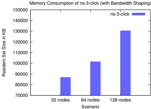
Figure 11: Average memory consumption of ns-3-click for running an IP Router configuration with bandwidth shaping.
