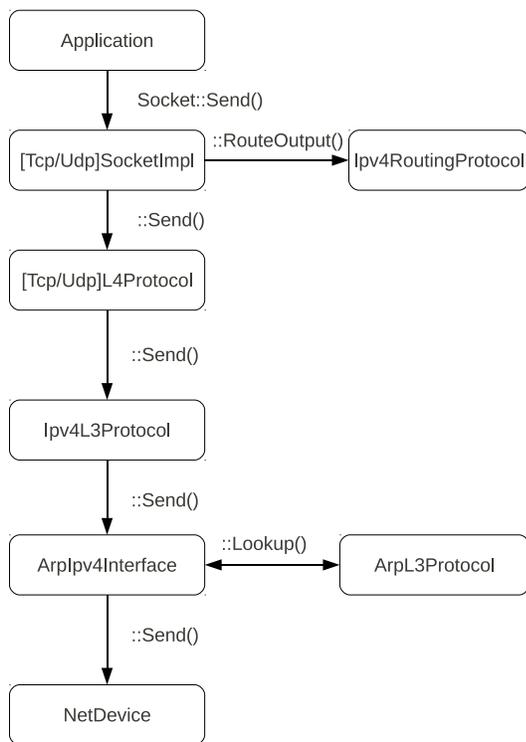
**Figure 3: Path of a packet going down the stack in ns-3.** The packet flows along the downward arrows, via the method invocations indicated on the arrows, with queries being made to the routing protocol and ARP protocol at appropriate stages.
